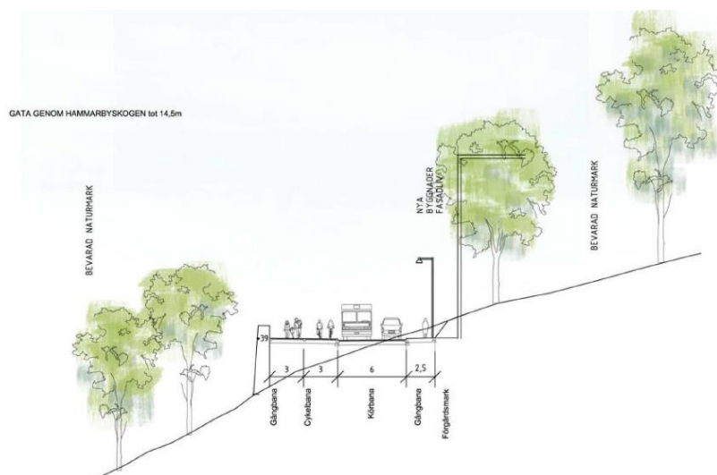
FIGURE 4. DEVELOPMENT OF HAMMARBYSKOGEN AND THE NEW ROAD (14.5 METERS WIDE) WHICH WILL CONNECT HAMMARBYHÖJDEN WITH HAMMARBY SJÖSTAD. TOVAT ARCHITECTS AND PLANNERS, 2016, 37.
