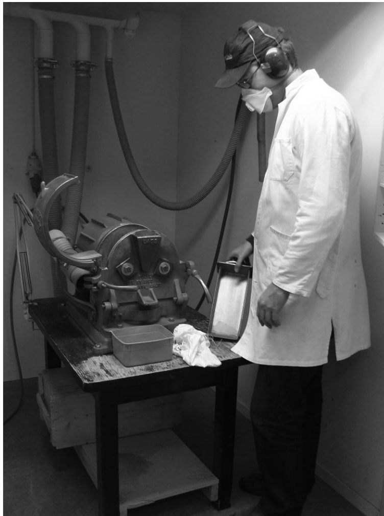
Crushing rock samples in preparation for cosmogenic exposure dating. Photo: Helena Alexanderson.
