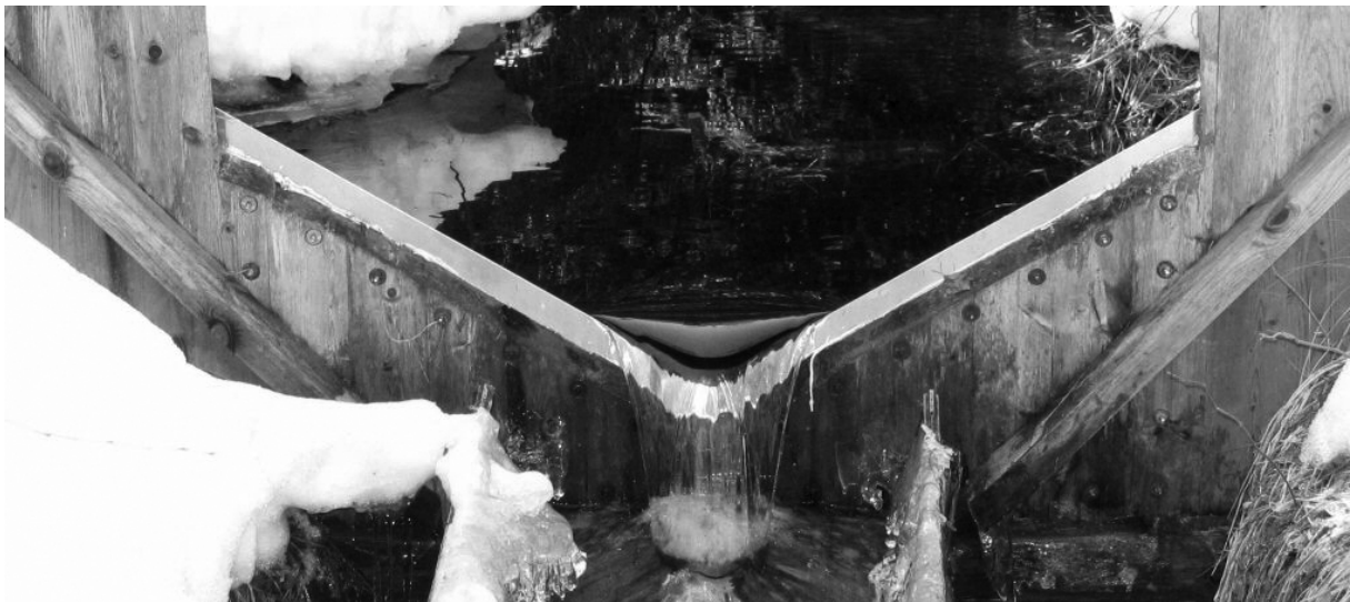
Runoff measurement station (V-notch weir) at the outlet of the Östfora catchment. Photo: Jan Seibert.
