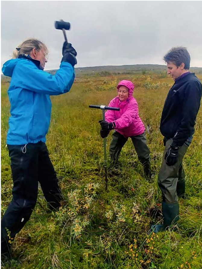
Britta Sannel from the HWP unit hammering down a Russian corer into partly frozen peat in Finnmark, Norway. Unit member Marit Hichens-Bergström is holding the rod and Master student Brittany Tarbier is watching. Photo: Stefan Wastegård.
